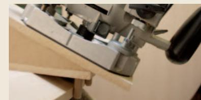
was made using the fence mounting rails for the router this re-adjustment would be quicker. Similarly the bevel angle could be made to be variable. I made mine fixed at 23° as it was very quick to make from MDF, and the number of times I'll use it will probably not justify the extra work involved in making an adjustable version.
