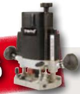
Although this is a slightly tricky project, it doesn't need a lot of router cutters. I chose a **two-flute 3.2mm diameter straight cutter** (1) for all the glazing slots. The slots were all done in one pass so care is needed to avoid breakage. You need to do a repeat pass to loosen the tightly packed chippings that will jam the slot.
