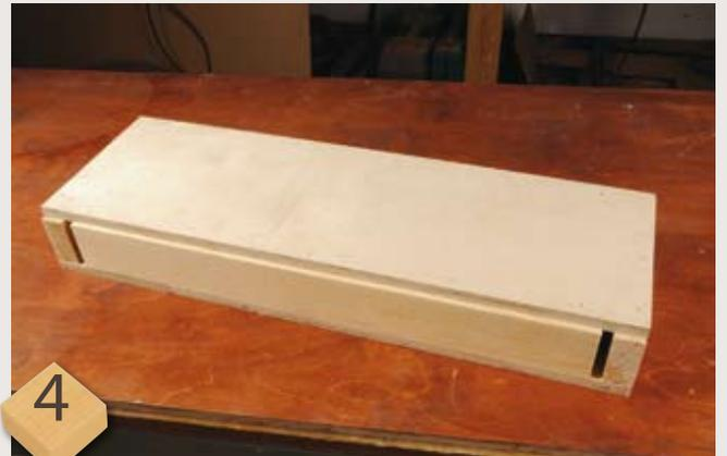
Cut two pieces of 9mm or 12mm birch ply to fit inside the base pieces and four offcuts of softwood all glued together to create a box around which the facings will be glued. The top piece of ply is narrower to create a rebate for the cabinet back panel. The softwood and plies must be flush all round apart from this – check with a square after clamping up
