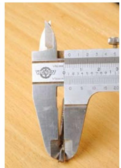
Measuring the cutter diameter
