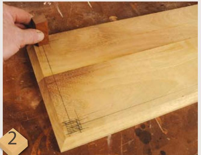
Having machined the bevel, mark out the positions for the four corner glazing bars and the slots for the polycarbonate glazing. This setting out is crucial and needs to be done using an offcut of the glazing bar to get the marking out correct. Put marks on the top side to show where to start and stop the slots when machining on the router table
