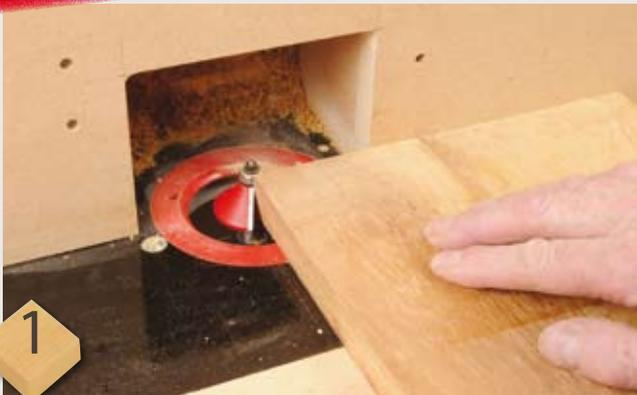
Decide what size the cabinet needs to be – this is governed by internal height, width and depth sufficient to contain the trophies. Cut the cabinet top to size including the extra amount for the projecting edges. Set up a large bevel cutter in the router table and do the bevel edge in several passes to depth. In this case, you can alter both cut depth and width as you work towards the final cut
