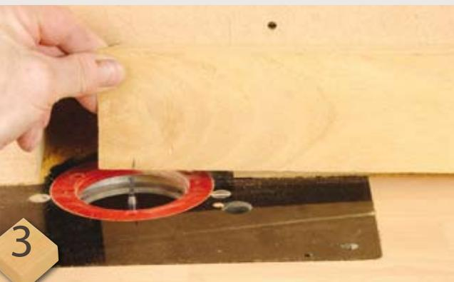
Machine up the front and side facings for the base including the glued on brackets for the ends. Use a mitre saw to create butt joints at the front corners, using the cabinet top as a position guide when marking out. Use 'drop on machining' for the glazing slots in both the cabinet top and the base facings. These slots must not meet in the corners as there will be location dowel holes there
