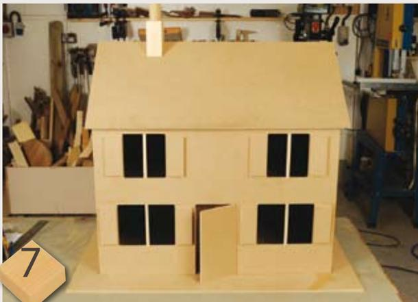
**7** Cut and glue a chimney stack in place and make a staircase from square section softwood and two thin strips of MDF, then install. Any mouldings can be fitted in the rooms as well. The windows need glazing bars and a front door. The front can be hinged or held on with swing-over clips. The dolls' house is now ready for painting and decorating, and lots of fun! ■
