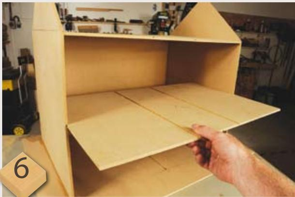
**6** Butt glue the outer walls together, and onto the baseboard as well. Dolls' houses are generally done without more complex joints because of the relative simplicity. Slide the floor, ceiling and walls into place with some glue brushed onto the edges first
