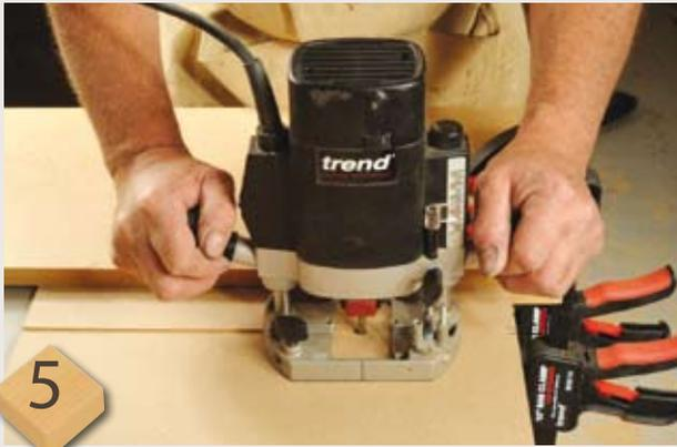
**5** Mark the floor and ceiling positions on the inside of the walls, and use a straight cutter and a router T-square to make shallow grooves for the floor and ceiling to slide into. Cut and fit the floor and repeat the grooving operation for the inner walls, ensuring you copy the marks across between components so the grooves will line up correctly. The walls will need door openings and the floors stair access, of course
