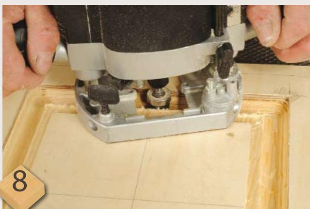
**8** The door is cut to size and a template made for the bearing guided face moulding cutter (see Router Class in WPP43 for more on template working). Make sure you use an offcut in the middle for support and keep the router tight to the edge of the template and machine at an even pace. The template is pinned to the door blank and the blank sits on a rubber router mat. The edge has an ovolo shape routed on it. Finally sand, apply a finish, and fit the hooks, hinges, knob and a catch! ■
