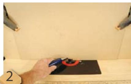
**2** and kickback occur at slower speeds, and you need the fence to stay put. If there is a bearing or shaft on top of the cutter you need to cut this area out with a bandsaw first. Your subfence is now ready and you can wind the cutter up or down while running. Trim away any fluffing or tearout at the outfeed side of the cutter with the router switched off.
