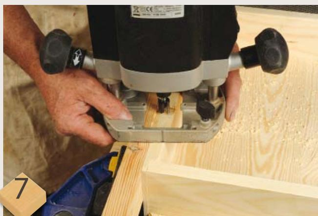
**7** Now cut the top and bottom to fit when the side pieces are in place. All components can be sanded and glued and pinned in place. For simplicity, the hinge recesses can be machined to the full depth of the folded hinge into the cabinet carcass, and simply surface fixed to the door. You don't need a jig for just two recesses, but you do need to clamp a batten along the cabinet side to give more support for the router and fence
