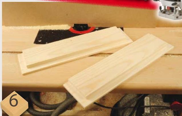
**6** The cabinet sides are also rebated so they sit along the sides of the back panel without projecting too far, for aesthetic purposes. Do this at the same cutter and fence settings
