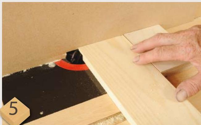
**5** Use a tenoning cutter, or a 19mm straight cutter with a through fence in place to machine a rebate on the ends of the cabinet side pieces. Use a square cut push block behind for accurate support and to avoid breakout
