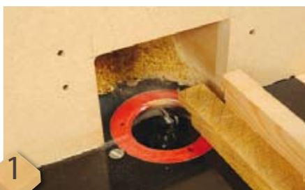
**1** marring the finish. Where a cutter will be partly behind the fence line, fit a sub-fence and start with the cutter well behind it. Switch on and push the fence back carefully until the cutter breaks through and is exposed enough for the cut you need. Keep hold of the fence and press the NVR switch to cut the power. It is best to keep hold of the fence for this, so have a friend switch it off for you. This is because snatches
