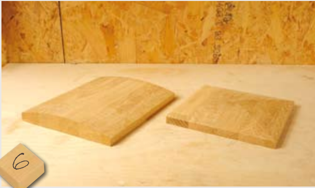
The left-hand example would suit a treasure type chest while the right-hand version, machined in both directions, would look good on a box
