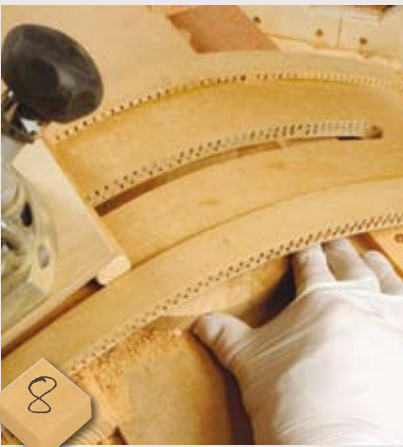
Now make repeated passes, turning slightly each time to machine a new area, until you have cut the full circle. Then pack up the workpiece to make deeper cuts until you have the full curve. I wore a latex glove to make holding the workpiece easier for turning and holding steady. Remember, your fingers must not be under the jig with the router running
