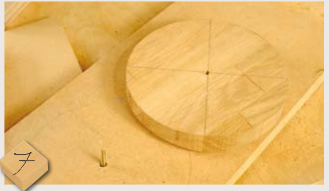
You can make a round lid by taking a square version and marking a circle on the underside, bandsawing it out and smoothing the edge carefully until fully round. Then mount it on a screw projecting from the packing board in the jig so it is just free to turn
