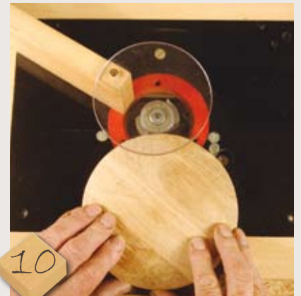
Machining the cookie jar lid rebate was done using a bearing guided rebate cutter with a suitable size bearing fitted. A lead-in pin ensures a safe run off into the cutter. Ensure the lid is turned into the direction of cut, or it may just become a Frisbee and fly off the table. Note the Perspex cutter safety shield over the top
