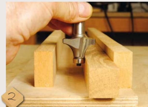
**2** The space inside the jig should be such that the component will sit in the jig with enough clearance to one side for the roundover cutter and bearing, in this case a 12.7mm radius cutter. It is important the cutter will not randomly catch on the side of the jig – although if this does happen the consequences shouldn't be very serious. Mark this position
