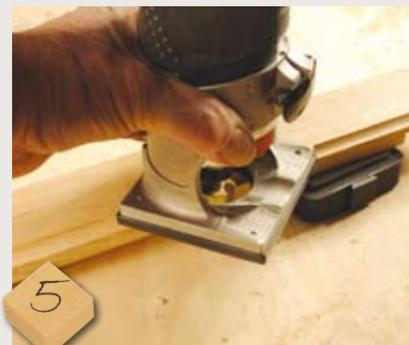
5 A small cove cutter is used to relieve the rather thick looking edge of the board. This is done from the opposite side to the dowel slots. Note the bearing must be able to run against the wood just above these slots or the edge will get damaged at this point and ruin the job
