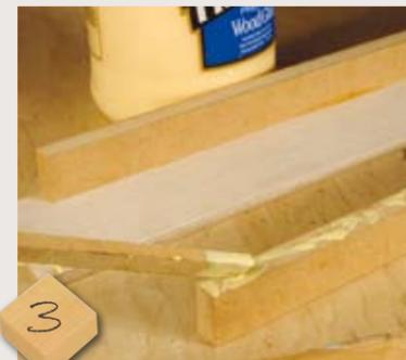
**3** Now you know the position of the jig's second side trim the base of the jig down on the saw and glue and pin the second MDF strip. This forms a U-shape. Ensure there is no glue at all in the internal corners
