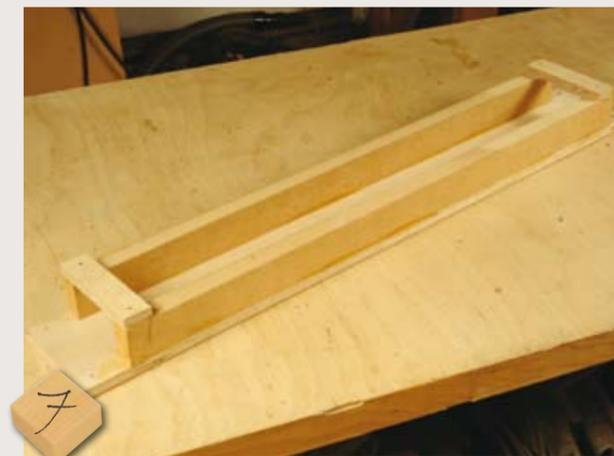
**7** The completed jig is very simple but it is being asked to do a very accurate job turning square stock into round dowel. Accurate preparation of the blanks is important for a good result
