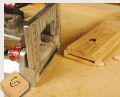
6 Now is the time to accurately cut all the components apart. The ends will be biscuit to the back board. This job is most safely done with a biscuit jointer. I used two No.20 biscuits as packers to centre the 0 size slots, slow plunging is needed to avoid any kickback
