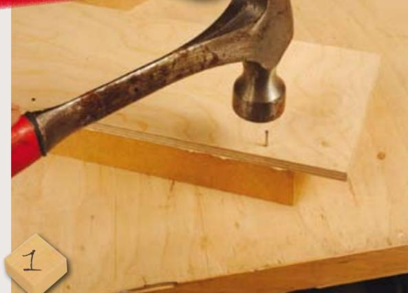
**1** Cut two strips of 18mm MDF or ply, slightly wider than the intended size of the dowel you will be making. The jig can be made longer to suit other projects... the principle remaining exactly the same. Glue and pin a strip of MDF along one side of the strip of ply, to create an L-shape
