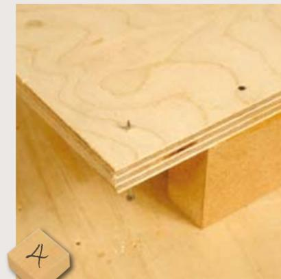
**4** To stop the jig slipping around, four panel pins are driven through the corners of the jig so the tips project through
