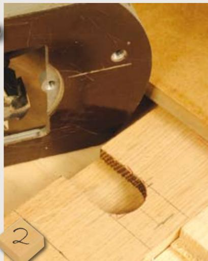
2 I used a 25mm tenoning cutter and a standard housing jig to guide the router. A second pass is needed to widen the slot by 2mm. Ensure you machine in the direction of cutter rotation, the other direction, climb cutting, can make the router run away and possibly damage the work
