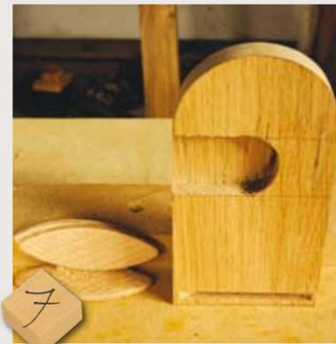
7 Cutting the slot in the end component requires care. Raise the component up on a single no.20 biscuit to get the correct height, and then use two biscuits behind the component, so the jointer doesn't foul on the bottom biscuit. Plunge slowly, and keep your fingers away from the cutting end of the jointer
