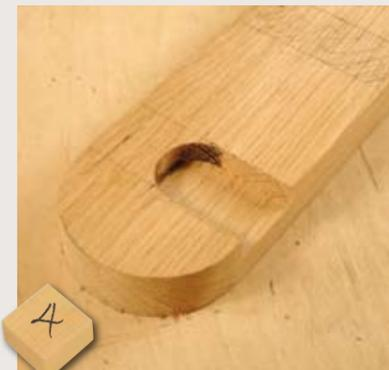
4 The end cheeks need rounded front edges. Mark the curves and bandsaw them close to the line. Obtain a smooth curve on the drawn line using a disc sander or a static-mounted belt sander
