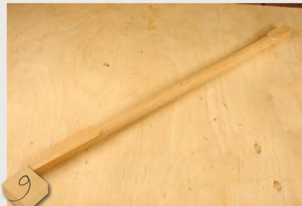
9 You should end up with a nearly perfect round dowel in your chosen timber. It will need a little sanding to iron out any tiny inaccuracies, and then it is ready to trim to length so it fits in the completed kitchen towel holder
