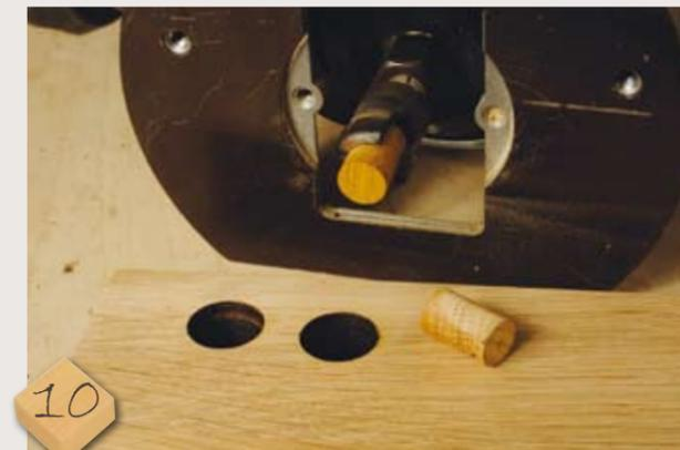
10 The fixing holes in the holder can be plugged neatly for a discreet appearance. I found the plugs separated completely after being cut and though there was timber burning in the waste side after the cut, the plugs themselves were fine
