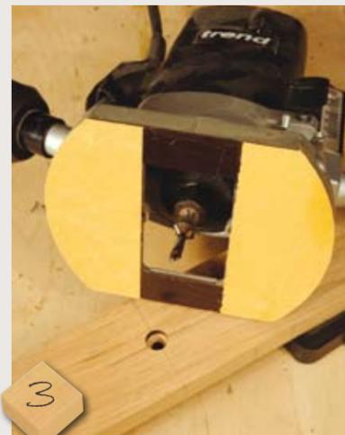
3 Drill and countersink two holes for mounting the holder using the router with abrasive spray-mounted on underneath to stop the router slipping around. The holes are cut from the face which does not have the slots cut in. I used proper counterbores rated for router use
