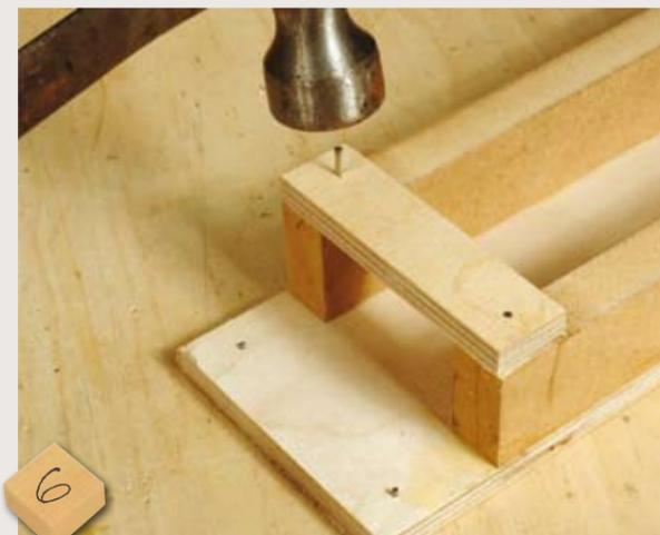
**6** A narrow strip is pinned on at each end to stop the router over-sailing. It also prevents the cutter from contacting the clamps when they are holding the blank in place
