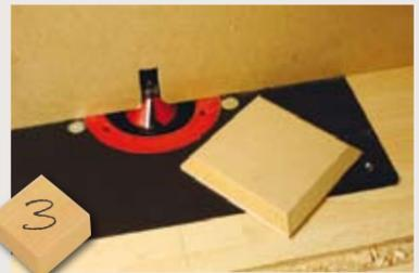
**3** The short legs are simply recycled bed legs with the castors and sockets removed. The screw threads need to go into thick enough material so we need to make special pads to give that extra thickness. A bearing-guided bevel cutter is used in the router table, with a breakthrough fence, to bevel the edges of the pads the legs will screw into. Note the slot cut into the breakthrough fence to allow the bearing to pass through when the fence is pulled back on to the moving cutter
