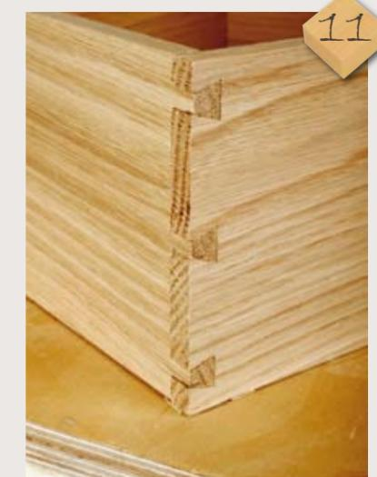
**11** The three pins look neat and even enough, but the acid test is always that the joints are a neat fit, and that they push together with just a tiny bit of resistance? After several trial attempts and learning how to get the best from the setup, here is quite a respectable joint
