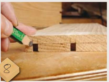
**8** To cut the other half of the joints, carefully transfer the slot positions to the front and back boards ready to create the pins. The marks are then transferred up the external face of each board onto the face of the workpiece which will be visible on the outside of the drawer box
