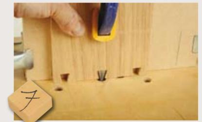
**7** Mark the sub fence to line up the workpiece edge so the end slot is cut in the right place. To do the other end slot, flip the workpiece around and line it up to the original mark. Make a second mark on the sub fence for machining the centre slot. You should now have three evenly spaced slots forming two dovetails and two narrow half dovetails at the ends
