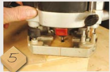
**5** Use a small router and a standard 6.4mm straight bit or a spiral router drill bit if you own one, to drill a hole in the centre of each pad. Mark the centre position first and set the speed to the lowest, and aim on to the marks, drilling deep enough to take the threaded rod on the leg. Now, simply wind the leg into the hole and the thread should bite and cut its way into the MDF and form a solid fixing
