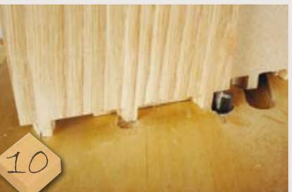
**10** Now, swing the fence to the opposite angle and machine the other side of the pin shoulder and then keep machining all the waste out between the pins. It really helps when doing this to clearly mark up your waste beforehand with hatched lines. The last shoulder is at the outside and you should be left with three, evenly sized, evenly spaced pins
