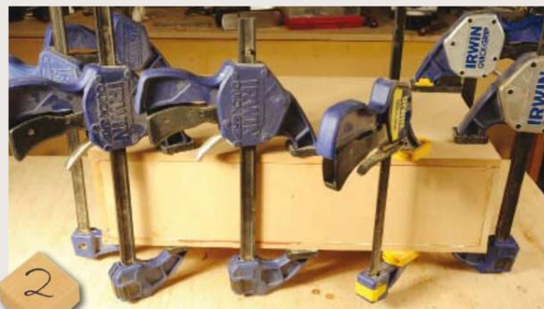
**2** Butt joint all the components together using PVA glue. Ensure all the edges are flush. Use plenty of clamps to hold it tightly so the excess glue is exuded, and wipe off the surplus. For this task, butt joints are quite strong enough
