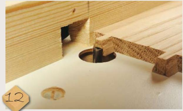
**12** The drawer needs a base, of course, but without losing too much interior space. I opted to run the 6.4mm base slot right in the middle of the bottom pin and did so without any problems with drawer integrity. Rather than doing stopped grooves it is easier to run right through. Once the drawer is assembled the little slot can be plugged with a matching plug
