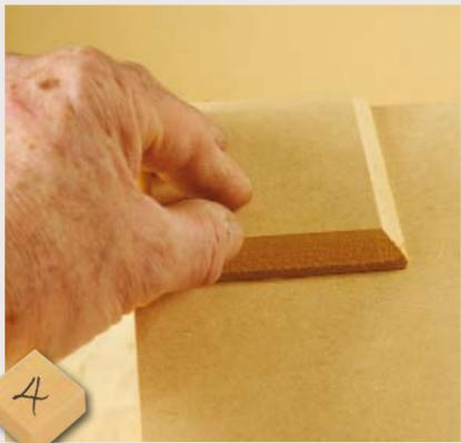
**4** Rub the glued blocks into place, lining them up with the edges of the carcass, and leave to set for some time as screwing the legs in could loosen the bond if not set properly. I was in a bit of rush and that's what happened to me!
