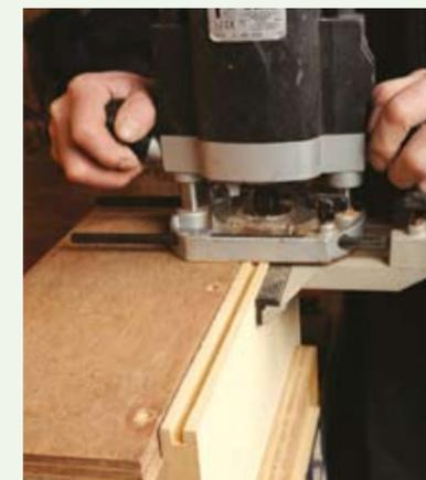
Edge slotting with an L-jig
