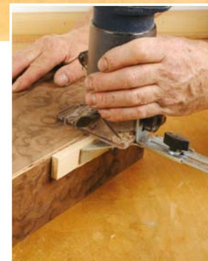
Machining to fit stringing using a trimmer and a straight fence
