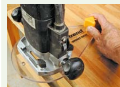
7 Slot cutters can be used to fit other more unusual biscuit components
