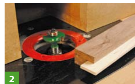
2 Machining slots for loose tongues
