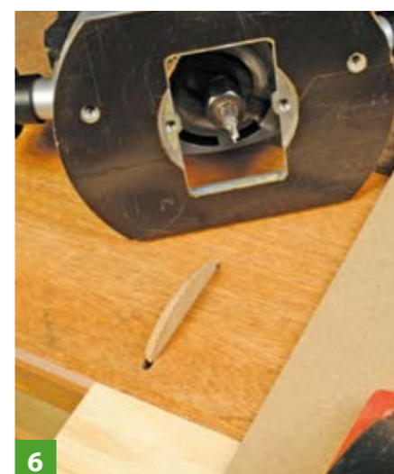
6 A 4mm straight cutter can create mid-panel slots
