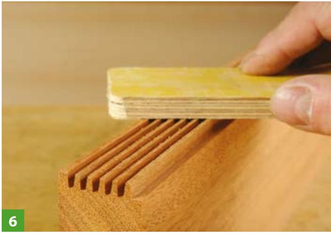
**6** The cutting action of a joint made with a fine finger cutter creates a lot of fine fibre strands on the edges of the fingers. In order to assemble the joint so it closes properly, it is necessary to dust and de-fluff the fingers using a medium abrasive rubbed along the edge of the joint halves, then blow away the dust.
