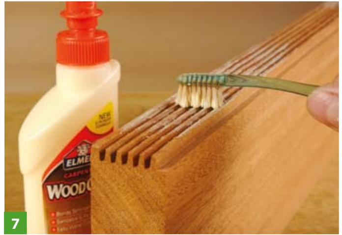
**7** Following on from that the gluing technique is important. If you dispense glue straight from the nozzle it will overload the joint with glue and the joint will not close properly, however much clamping pressure you apply. Instead use a brush and apply glue lightly to the tips of the fingers on both halves. Once the joint closes the glue will spread sufficiently to create a good bond. Do not delay assembly so the glue remains wet.
