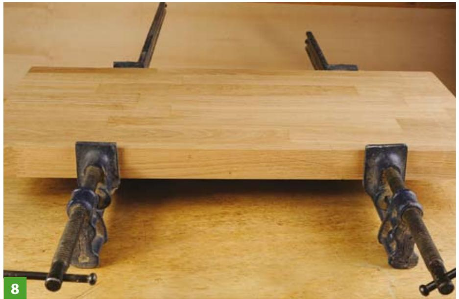
**8** Clamping glue jointed boards together has to be done correctly so the boards remain flat. The best clamps are T-bar clamps which are heavy and more expensive than sash clamps. However, you can make supports to hold sash clamps upright on the bench. Place paper over the bars to prevent glue wetting the bars and causing rusting and iron marks on the timber. Use more clamps on top facing downwards to improve the flatness of the assembled boards.
