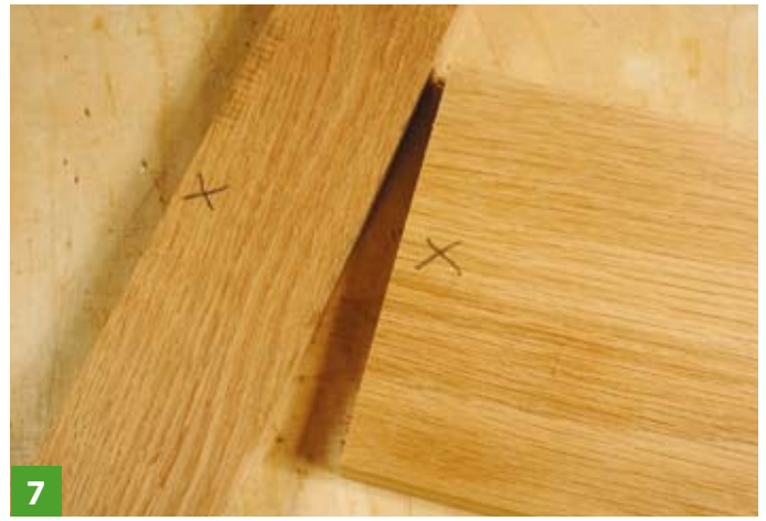
The crosses denote the face to be machined and on which edge
