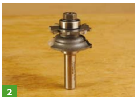
2 This cutter has to be reassembled when changing from profile to scribe
