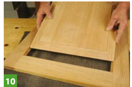
You should always check panel fit before assembly
