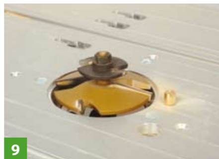
9 This panel raiser just fits in the table opening
