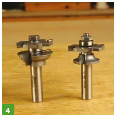
4 With two separate cutters it helps to have two routers
