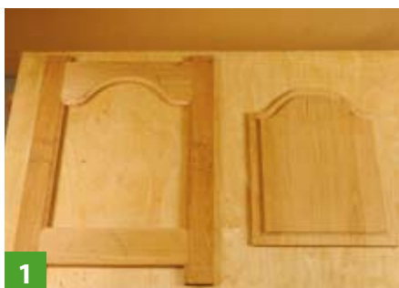
1 A typical frame and a matching panel for quick and easy construction
