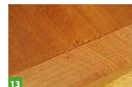
13 Tearout can result with the vertical type of cutter
