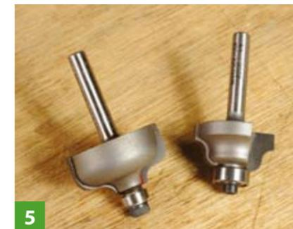
5 Ogee cutters create a flowing edge as an alternative to both cove and roundover
