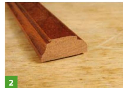
2 Both these profiles mould both edge and face in other words removing the arris
