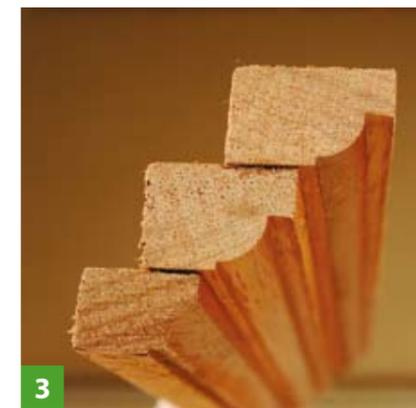
3 You can stack a variety of moulds and plain edged sections together and create an imposing cornice
