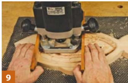
**9** Remove the centre of the dish moving the router anti-clockwise into the cut direction
