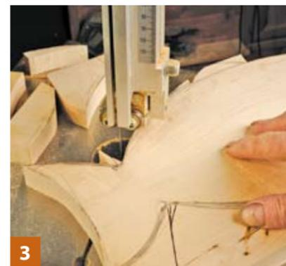
**3** Allow the bandsaw blade to follow your line and not deviate. Also, do not force the wood
