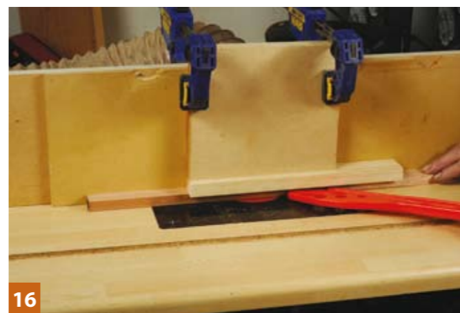
16 A 'semi tunnel' hold down
