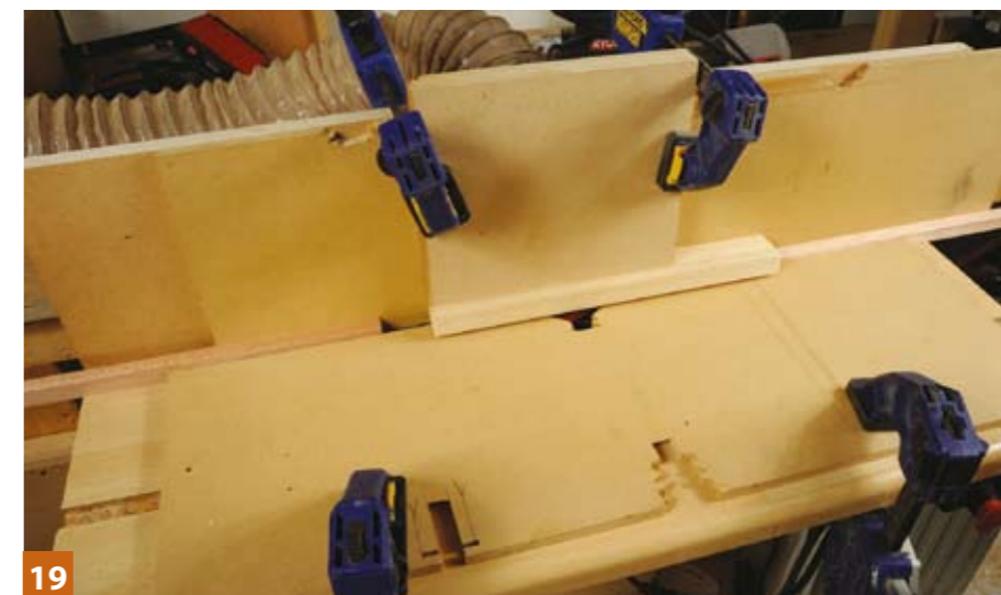
19 Although I have often shown pressure fingers in use I actually prefer continuous flat support as the sections to be machined are the same size
