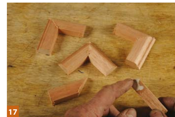
17 Make sure the joints will close properly and sit at 90°
