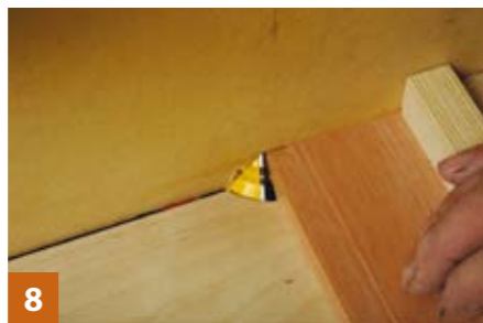
8 Making the second pass. A sub-table serves to maintain support right up to the cutter itself
