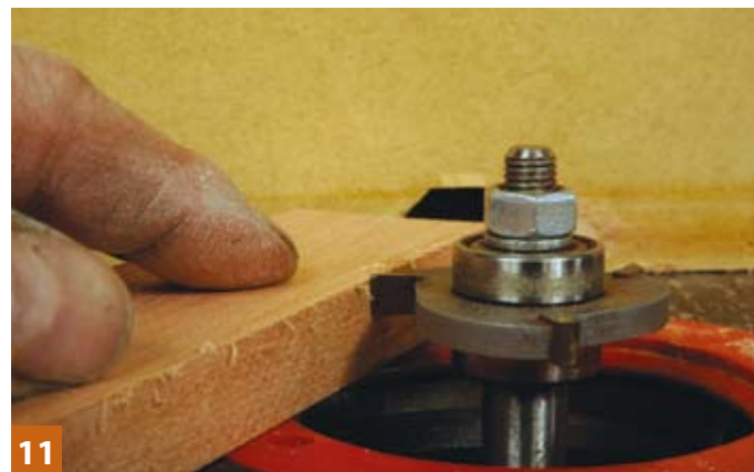
11 The tongue does not have to be 6mm but it is a good size for rigidity
