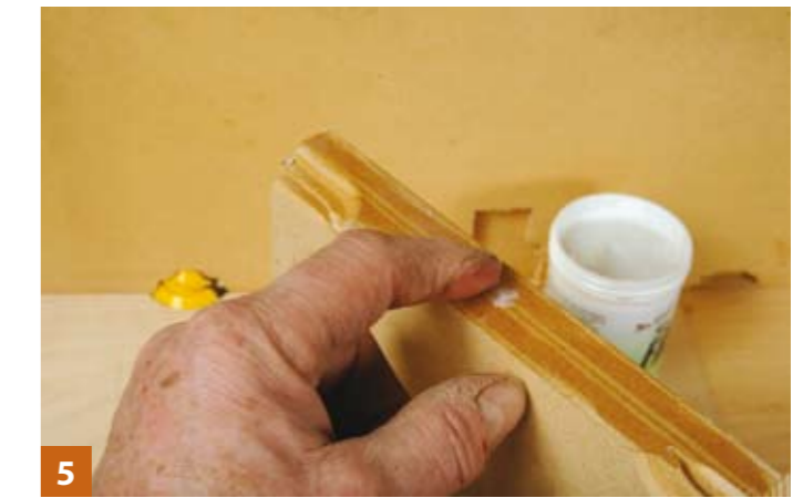
5 Unlike a mitre protractor a pushblock can be used with the fence in any position
