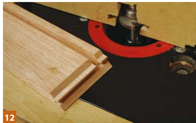
12 Again care is needed as you reach the end of the cut as the cutting edges pass through the joint
