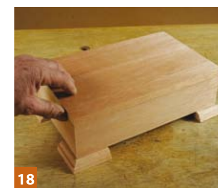
18 I positioned the feet by eye but you can mark them so you have lines to work to
