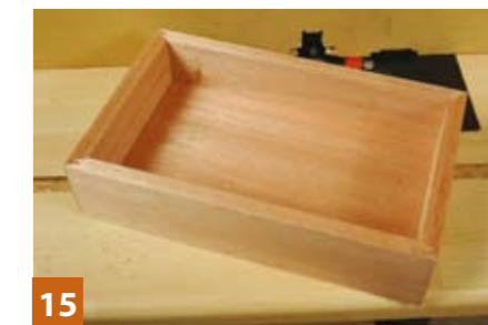
15 The box is now very rigid but needs the feet added
