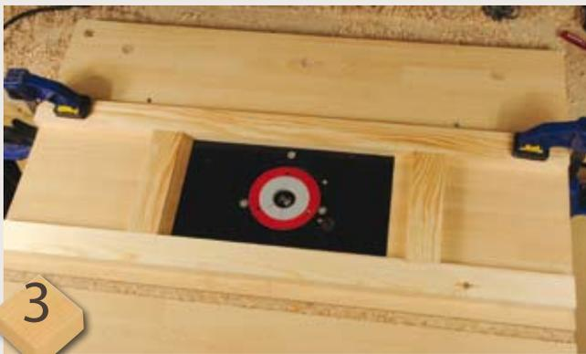
3 Fit a small straight cutter, say 2.5mm, in the router and lay the prototype door on the cutter so it is centred on the outermost vertical door line. Now clamp a batten running alongside the door. Move the door towards you so the cutter centres on the opposite outermost vertical line, and clamp that batten exactly parallel to the first one – this determines the width of the jig. Repeat the process for the length, cutting two battens to fit between the ones you have clamped
