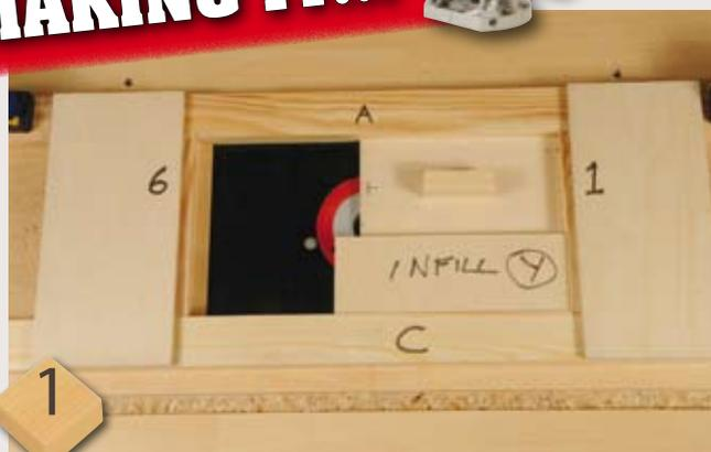
**1** The jig is already made and the door framing is the biggest challenge. Place the blank in the start position with infill 'Y' next to it
