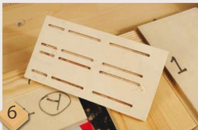
Repeat the sequence two more times, swapping 'X' and 'B' around, then remove 'X' and substitute 'Y' and you will end up with four matching lines of slots
