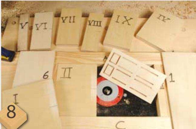
Using the series of crosswise blocks, machine all the slots using the drop-on technique for all of them. Working carefully, I managed to make a series of doors, each one taking under 10 minutes – if I got into the rhythm I'm sure it would be less. Once you master the thinking behind the process, it becomes fun and you can turn out doors until the cows come home, it's a job done
