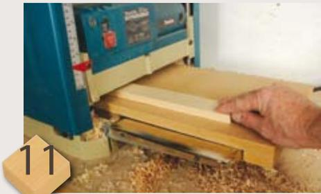
Thickening stock down thin enough for mouldings can be helped by fitting a false bed so you can go below the thicknesser's minimum capacity
