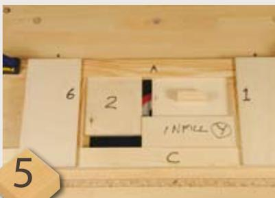
5 The first vertical line to be machined needs the numbered and lettered blocks shown here. The door blank has a grip handle glued to it to allow for drop-on cuts. This set-up makes the outer side of the topmost right-hand panel. Note the infill marked 'Y' which prevents sideways movement. To make the same outer line for the panels below, two more blocks and the infill are needed
