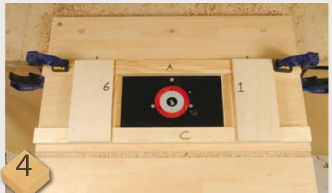
4 Ensure the jig is exactly square and glue and pin two pieces of thin ply on the outside ends of the jig – this will lock it rigid ready for the rest of the process. The numbers and letters relate to the door machining sequence. The machining problem we need to address is that we have to create six frames, in three sizes, in two vertical lines down the door. We need absolute control or the door blank will wander about and the result will be a mess
