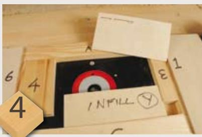
**4** The next slot is done using the next blocks marked '4' and '3'. The last slot in the line will be done with block '5'
