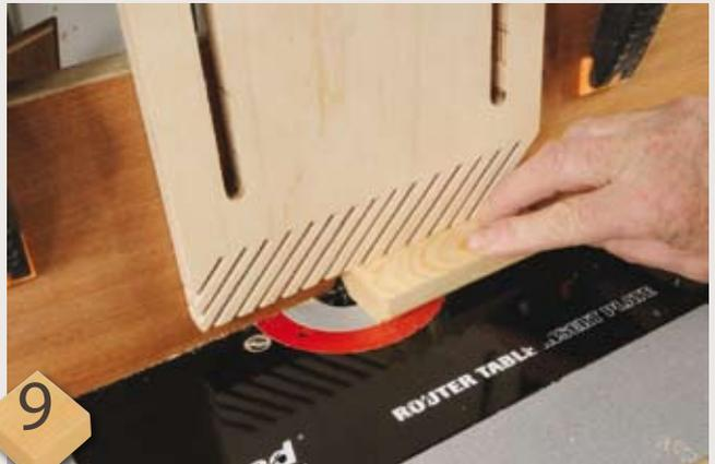
When machining small mouldings for the dolls' house, do it on the edge of a wider board and use sprung fingers and a breakthrough fence to give good, safe support. Then cut the moulding off on the circular saw and repeat the process to make more mouldings
