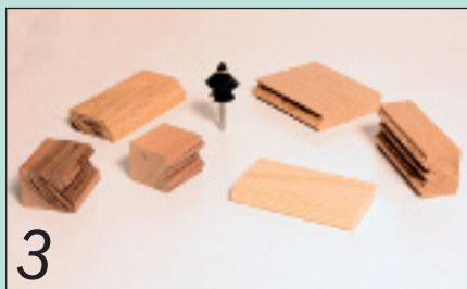
3 All these profiles in boards of different thicknesses were made with the T2940 cutter
