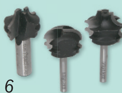
6 The multi-profile cutters on the right are from Wealden . The Trend cutter (left) has a 1/2in shank
