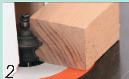
2 This is the full profile formed with the Wealden T2940 Classical Multi-profile cutter
